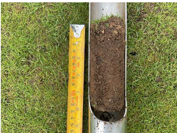
Photo 29: The soil profile on the green at The Leys appears reasonably healthy, but there is a persistent element of thatch in the upper zones.
