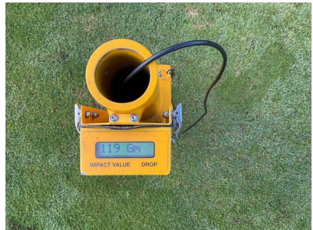
Photo 4: Encouragingly, surface hardness readings were around close to the projected target range of between 120-170 gravities and the green feels firm underfoot.
