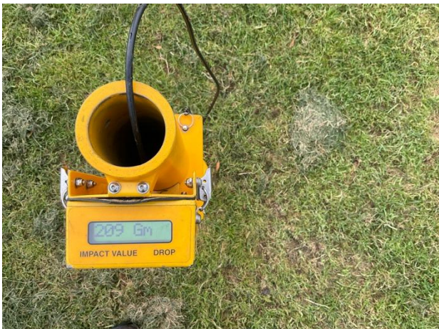
Figure 45: A random surface hardness reading of 209 gravities is quite high, but understandable given recent hot and dry conditions. The surfaces are deemed safe for use.
