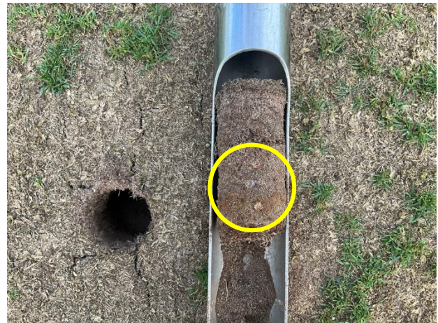
Photo 8: An inspection of the profile shows powder dry conditions, with water beading (circled) on the surface of hydrophobic soils.
